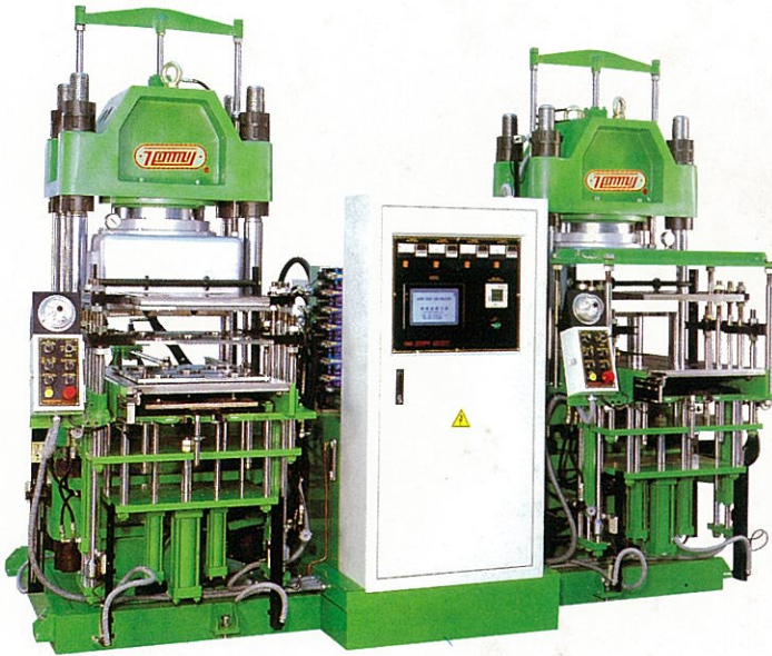
HEAT PRESSURE SHAPING MACHINE
